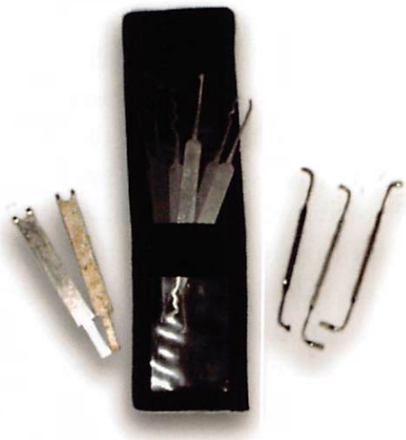
The Lab pickset that came free from ALOA a year or two back. Notice the nice thin tension wrenches which are great for tiny keyways. Notice also that some of mine are already broken!
