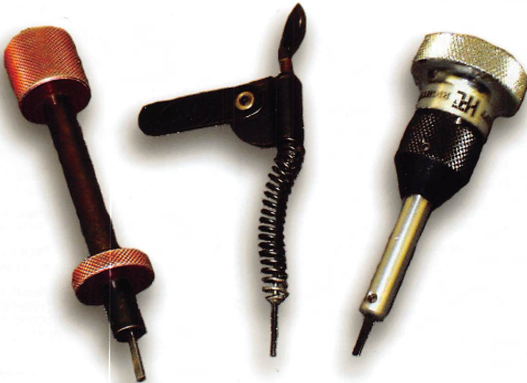
Three of the most common plug spinners on the market. Left to right, the Rytan, the A-1, and the HPC.
